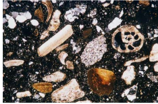
Figure 7: Petrographic analysis of the original bridge concrete showing presence of sea shells
