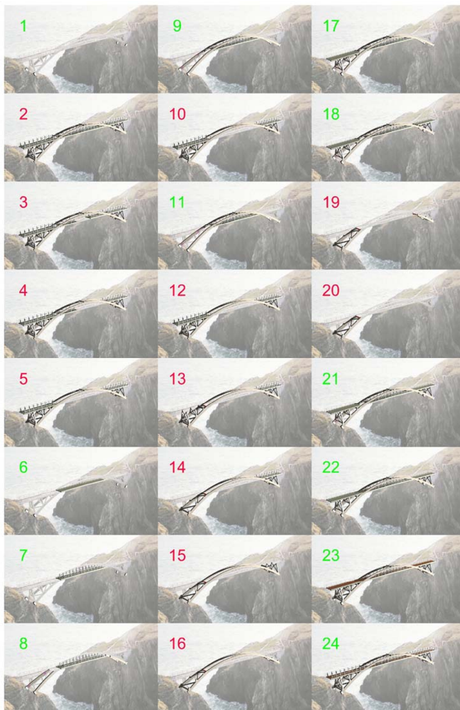
Figure 31: The integrated demolition and reconstruction sequence.
